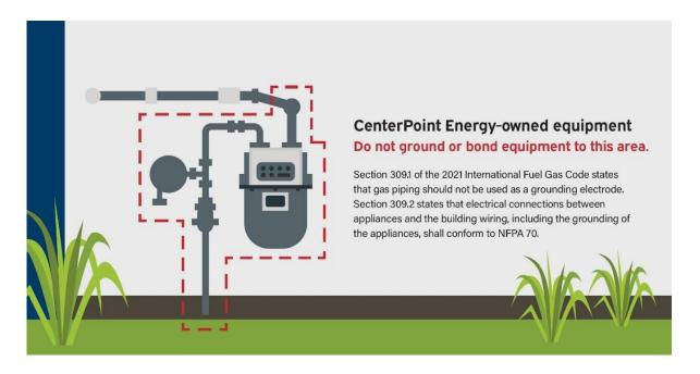
These safety hazards associated with improper bonding or grounding can result in lifethreatening circumstances.
