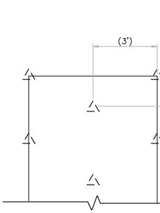
ANCHOR PATTERNS FOR SLOPES FLATTER THAN 3H: 1V
