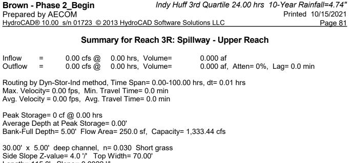
Length= 115.0' Slope= 0.0022 '/' Inlet Invert= 447.00', Outlet Invert= 446.75'
