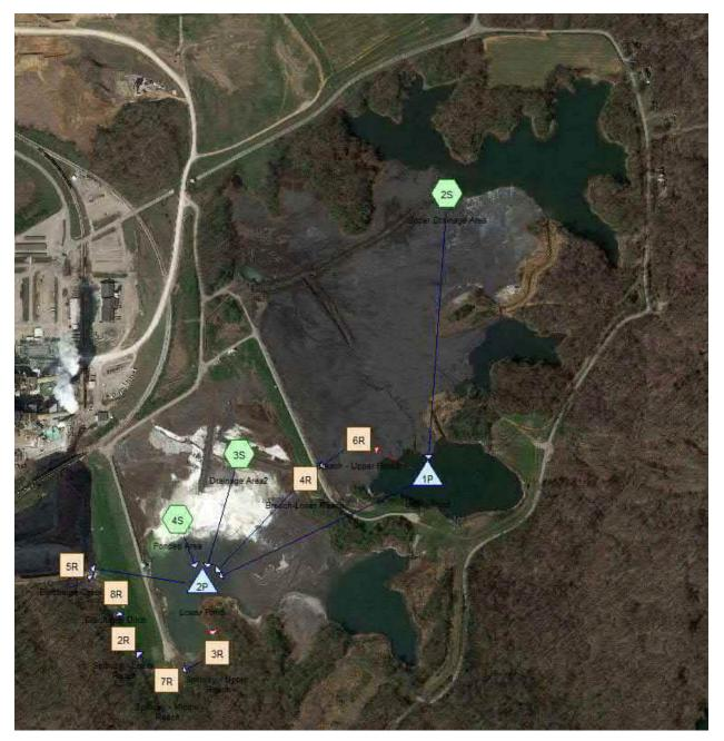
Figure 1. HydroCAD model schematic.
